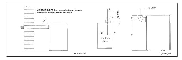
Adding a 90° bend shortens the total length by 1 metre. Adding a 45° bend shortens the total length by 0.5 metres.
