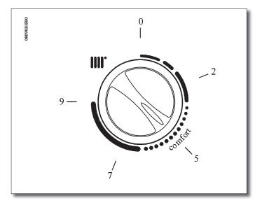
IMPORTANT: the range of heating flow temperature TM depends on the position of the jumper or switch T.RISC. (see paragraph 13). The maximum possible temperature setting is 85 or 45  $^{\circ}$ C.
