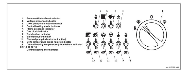
The lights 8÷13 display the temperature of the water in the central heating system (when not blinking).
