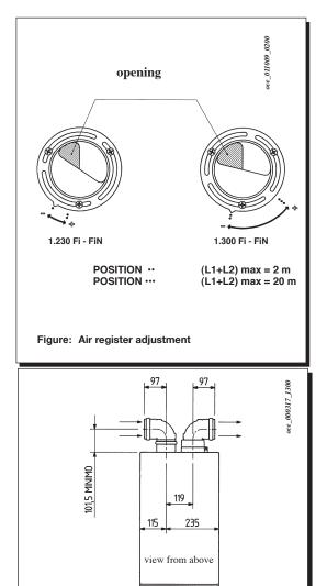
examples of installation with twin pipe horizontal ducts
